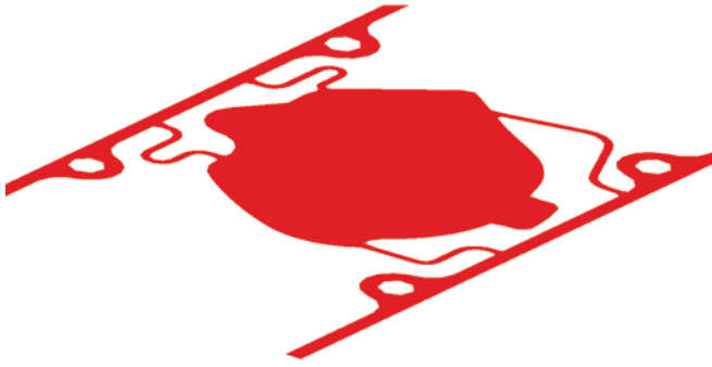
Fig. 2—Blank output with trim material and part carriers added
